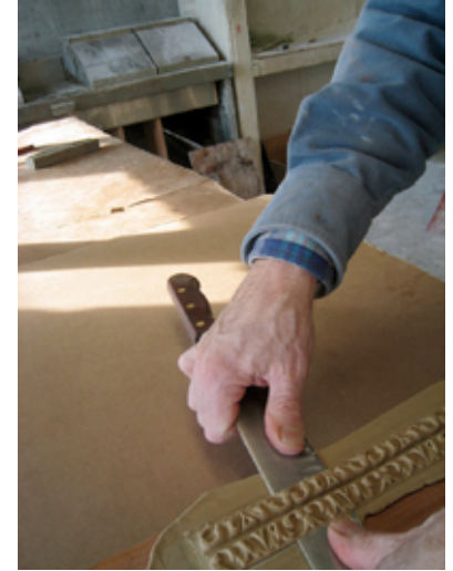
A thin blade is used to trim the composition ornament from the board and remove the excess compo.
