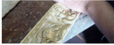
A composition ornament is carefully applied to the curved edges of a picture frame.
