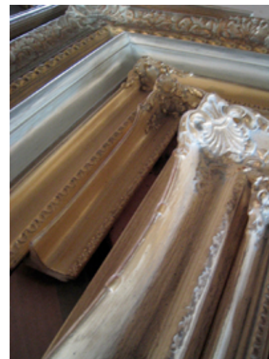
Frames ornamented with composition appear hand-carved but are less costly to produce and require less intensive labor than actual hand-carved frames.
