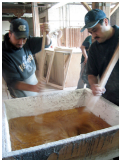
During production, the amber-colored pine rosin and linseed oil are heated and stirred
